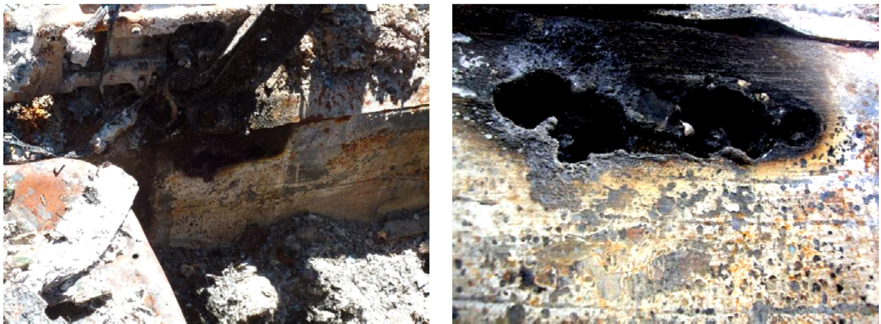
Figure 3.1-5. Holes in the Tunnel Section of the Battery Compartment Produced by Arcing
