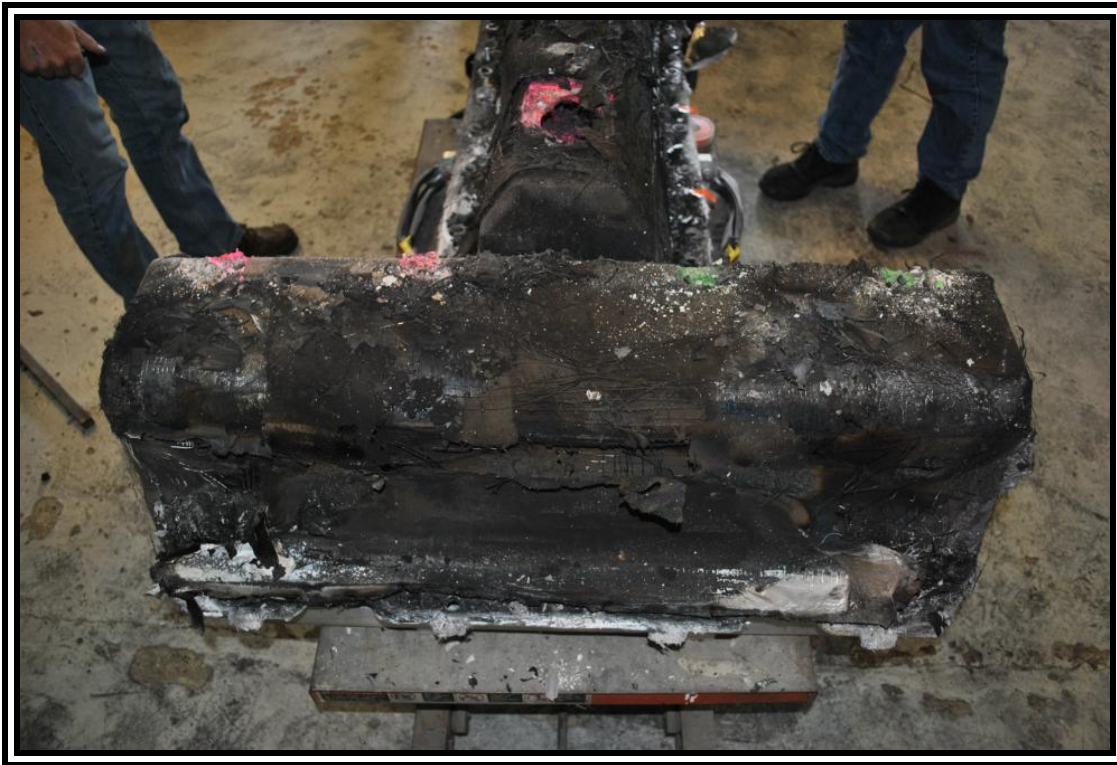
2011 Chevrolet Volt, rear of high-energy battery pack
