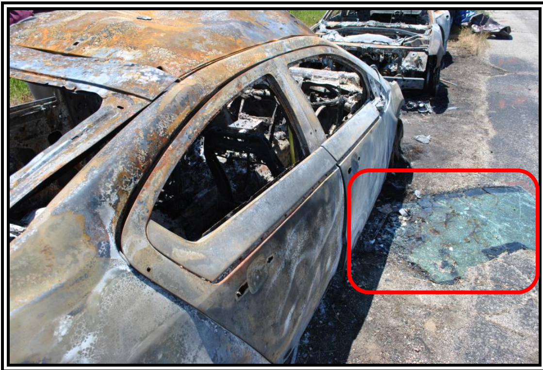
2011 Chevrolet Volt, displaced windshield glass laying face up
