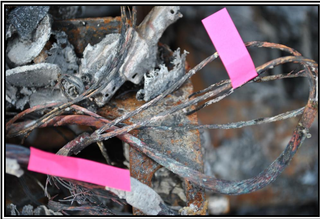
2006 Ford F150, intact fusible links to the alternator
