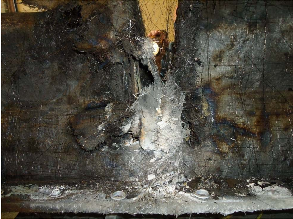
Figure 3.1-4. Battery Cover Damage at the Impact Location
