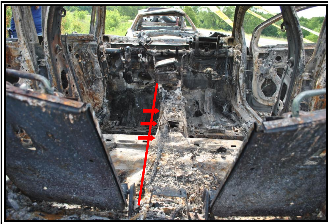
2011 Chevrolet Volt, observable 'radius' of the center tunnel
