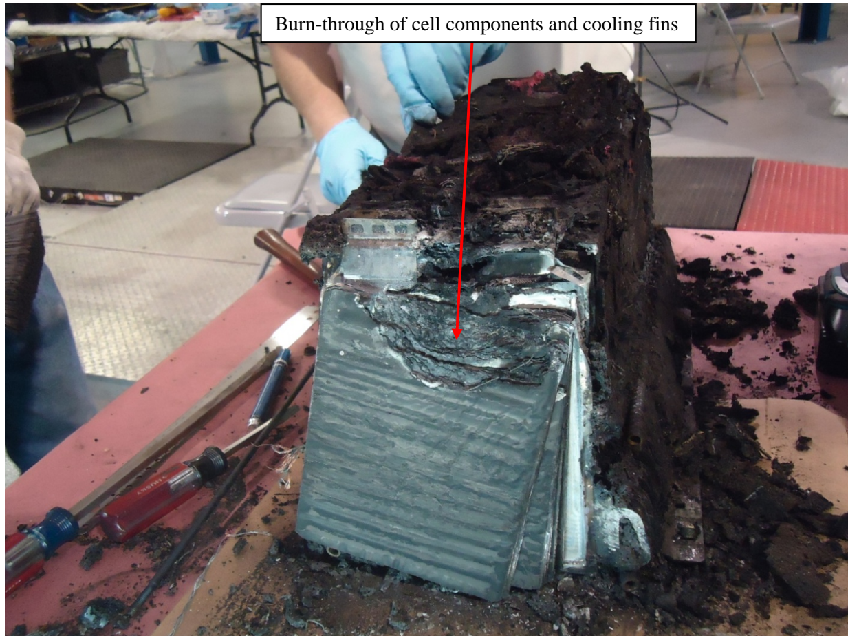
Figure 3.3-13. Remains of Cells 188–197 (“V” pattern)
