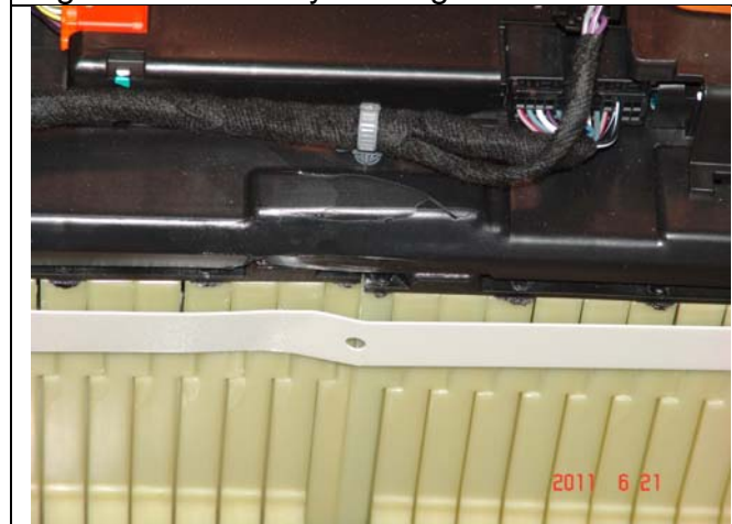
Figure 2.01 Battery Damage from Test 7385
