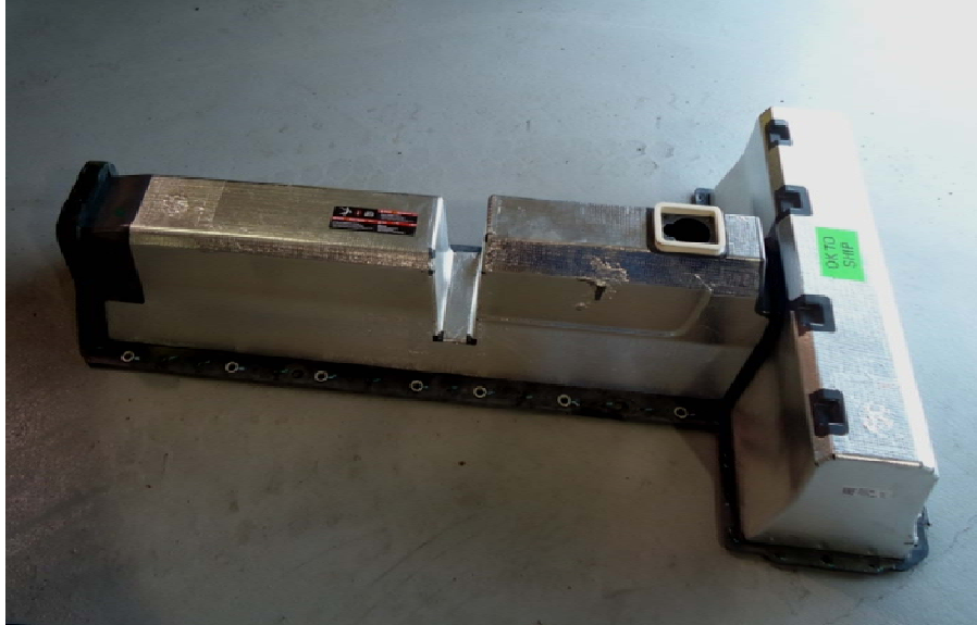
Figure 3.1-1. Fiberglass Battery Cover (new)
