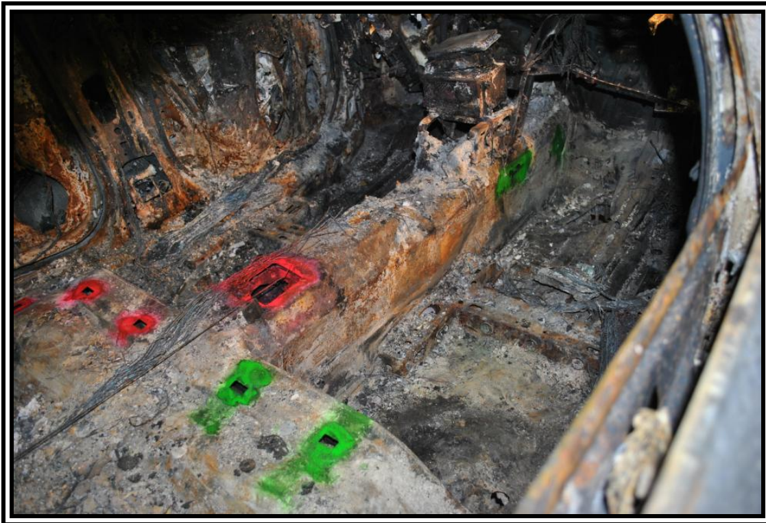
2011 Chevrolet Volt, GM paint marking of tunnel and battery
