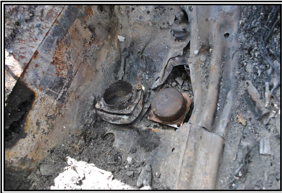
2011 Chevrolet Volt, passenger's side upper airbag module and exemplar module on passenger's side floor
