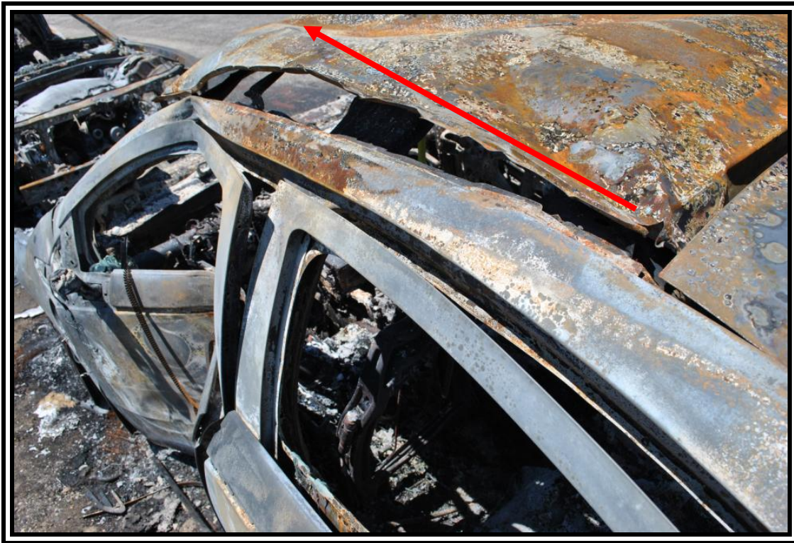
2011 Chevrolet Volt, dislodged roof sheet metal showing rear lift cylinder trajectory
