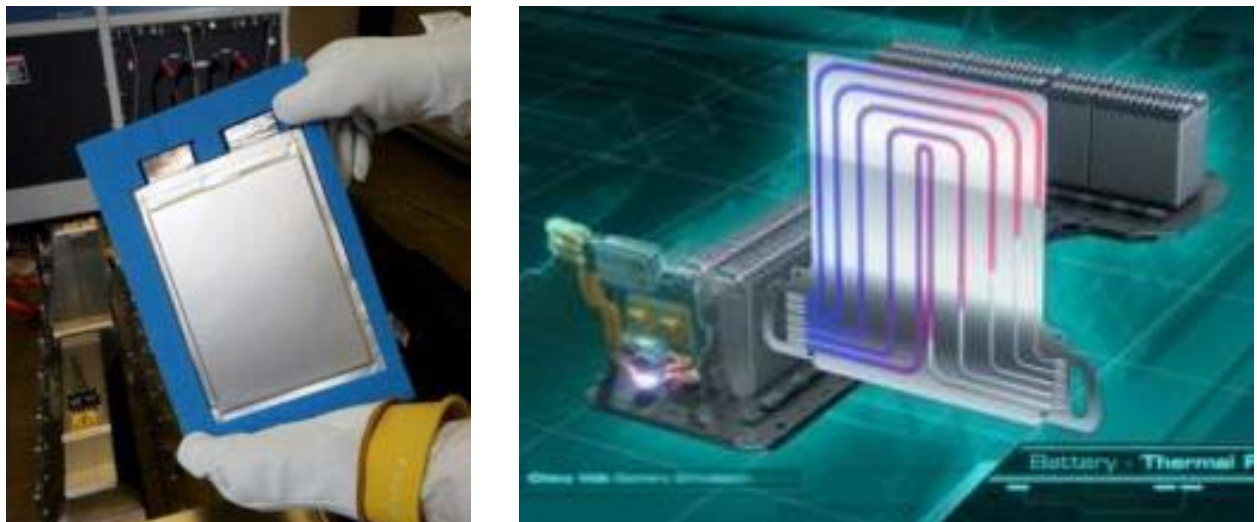
Figure 2.2 LG P1 Cell and Cooling Fin
