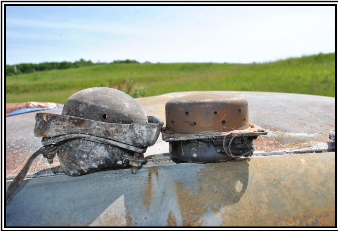
2011 Chevrolet Volt, comparison of the recovered airbag module to an exemplar
