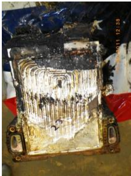
Figure 7.9 – Photograph Showing Cell Level Damage within Module 3
