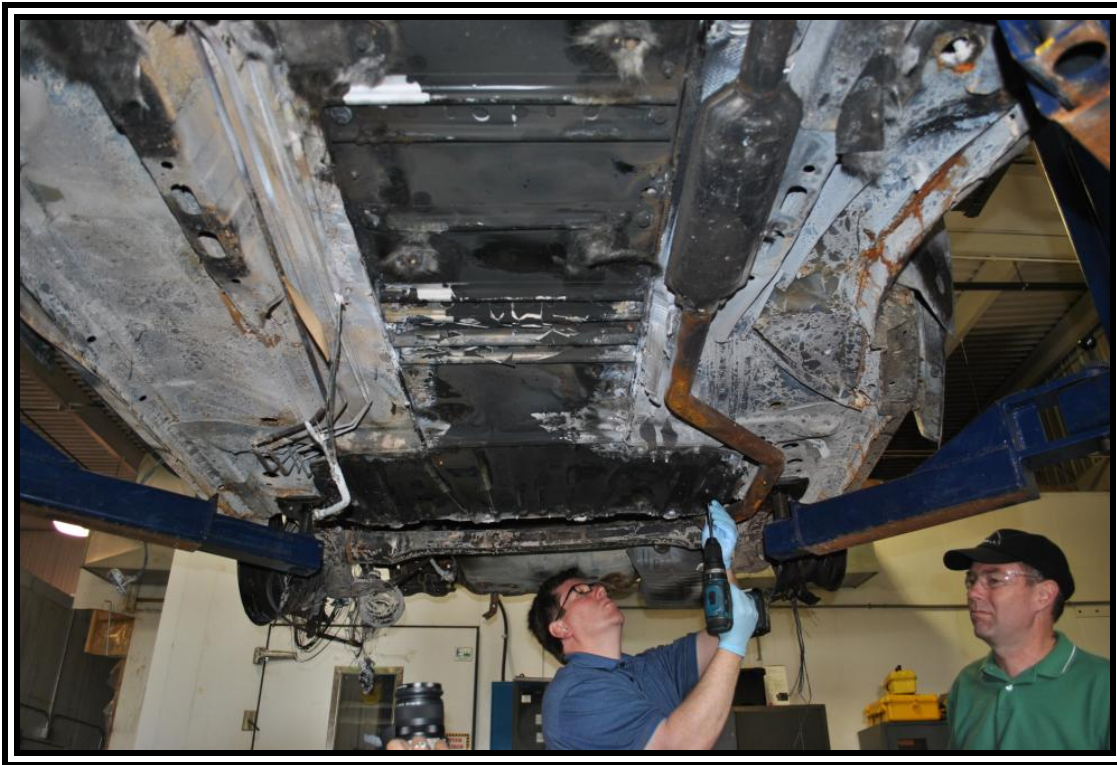
2011 Chevrolet Volt, initial high-energy battery removal
