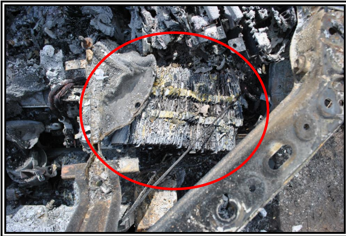
2011 Lexus RX350, driver's side mounted battery
