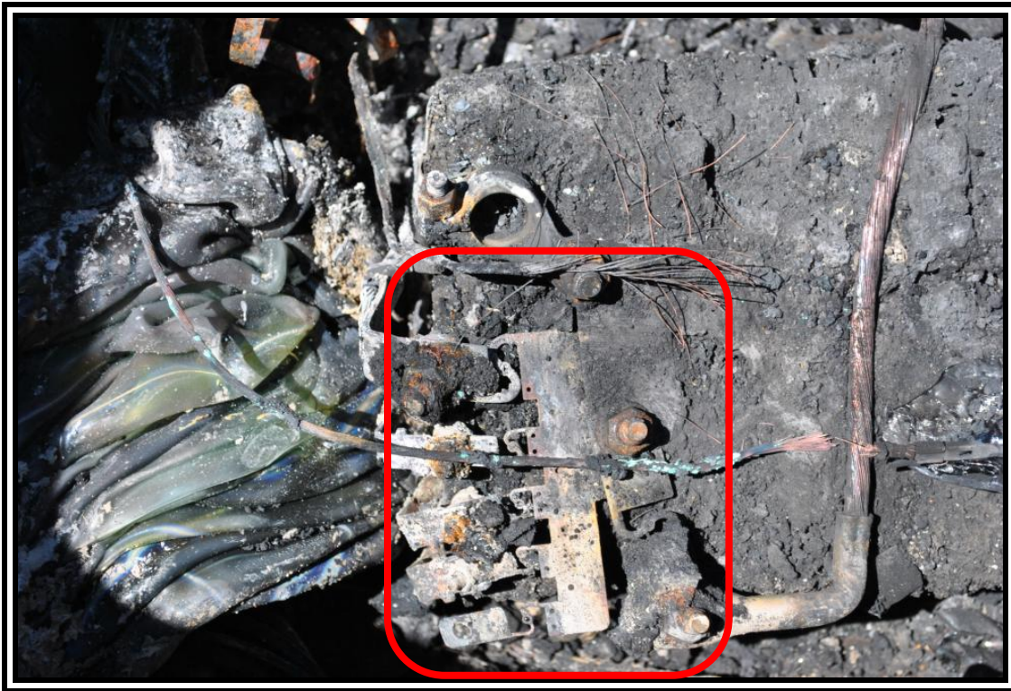
2011 Chevrolet Volt, intact +12vdc fuses at the battery
