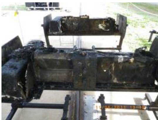
Figure 7.8 – Photograph of Batteries from Tests 1 and 2 (Battery from Test 2 is closest to the photographer)
