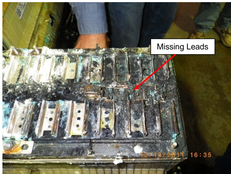
Figure 7.17 Fire Damage to the Bus Bar Leads
