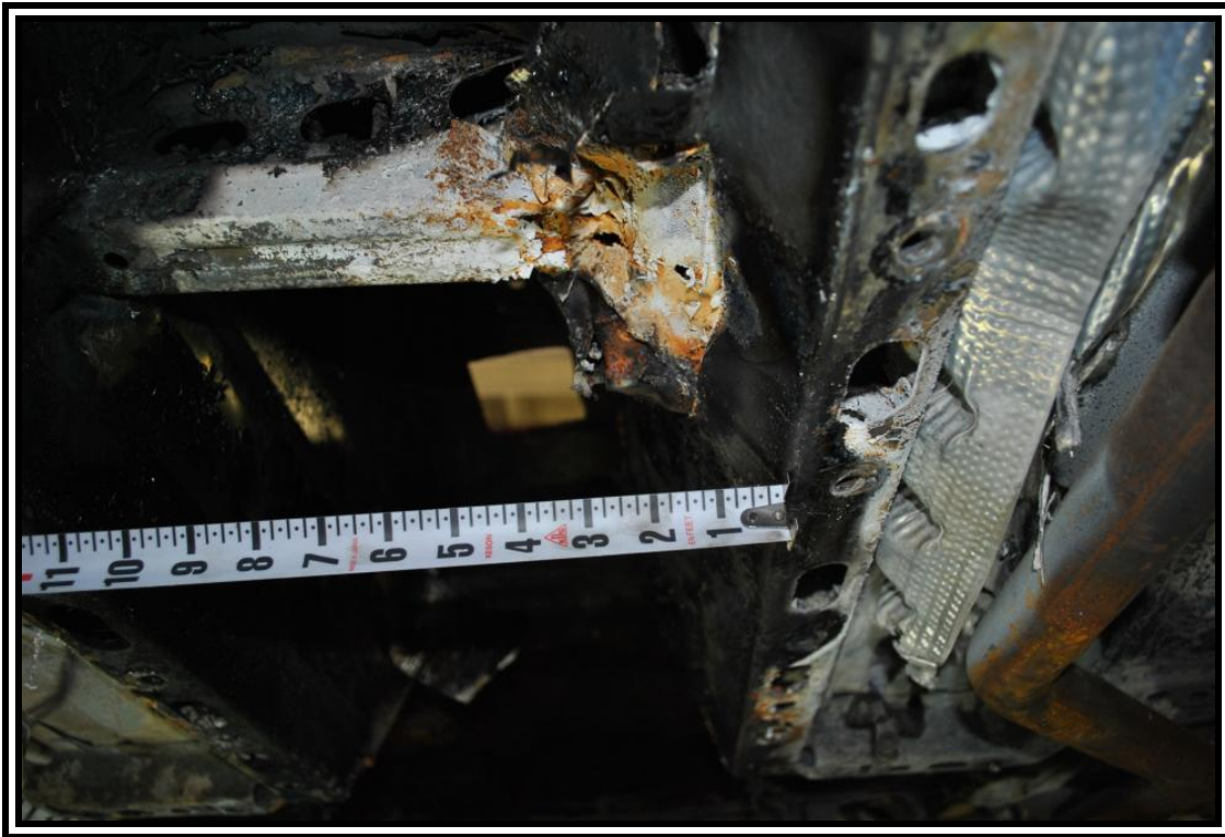
2011 Chevrolet Volt, measurement of intrusion into the battery pack tunnel
