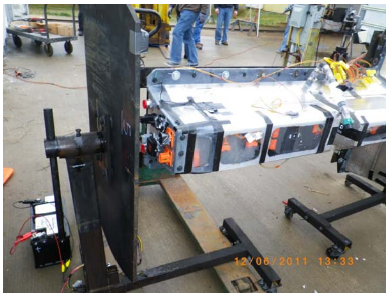
Figure 7.13 Test 5 with the Battery at the 270 degree orientation
