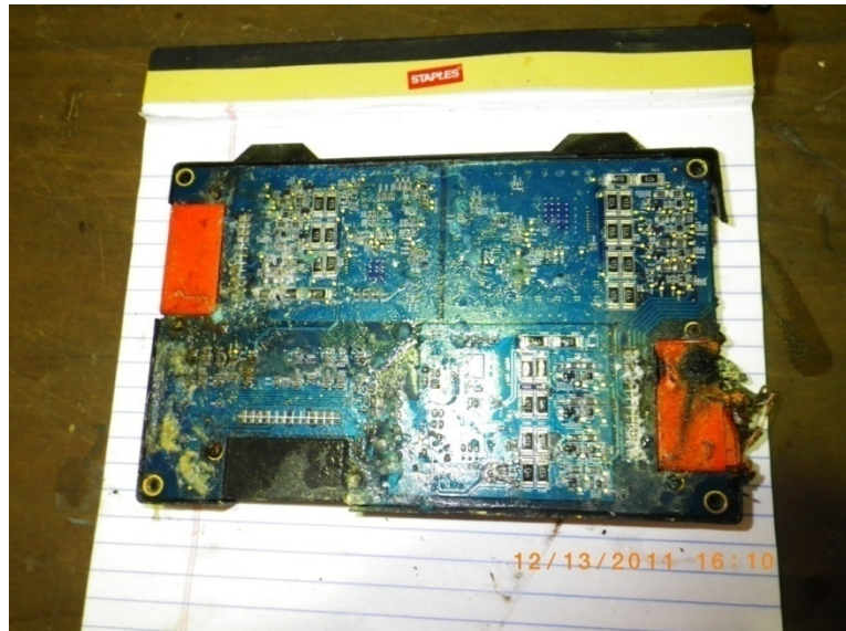
Figure 7.16 VTSM 3 – No Apparent Fire Damage
