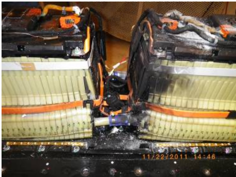
Figure 7.15 Arcing Damage to the Front of Module 2
