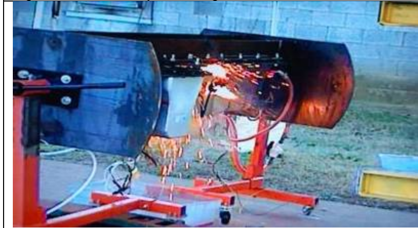
Figure 5.04 Battery 3 Arcing Event
