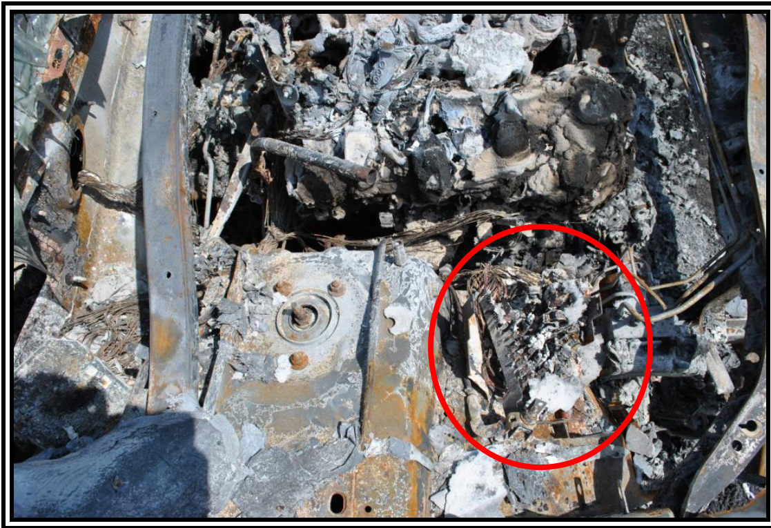
2011 Dodge Charger, passenger's side engine compartment power distribution panel
