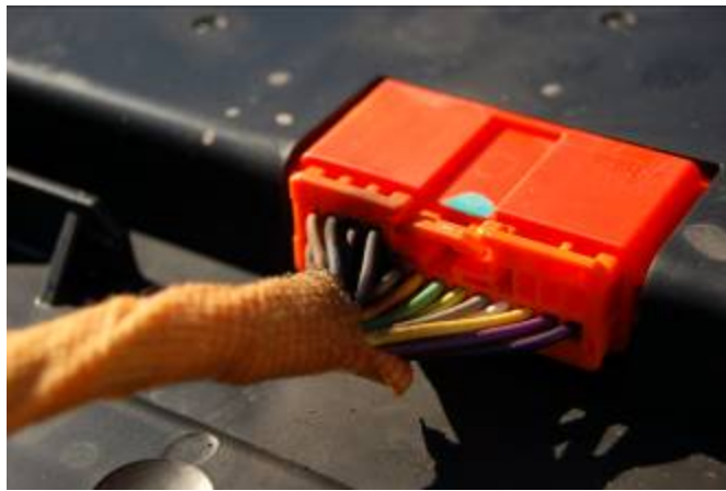
Figure 7.12 Discoloration of wires and orange jacket
