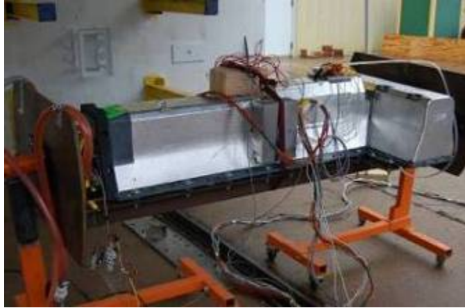
Figure 4.4 – Battery Cradle with Engine Stand & Battery
