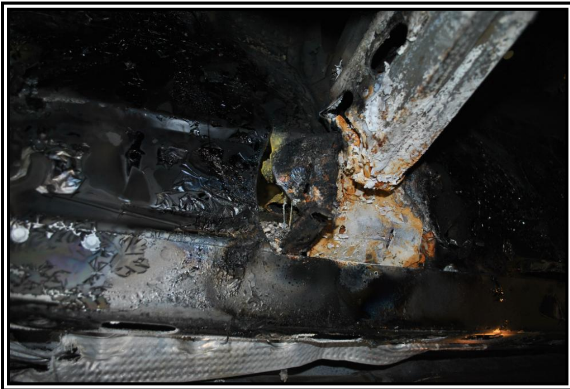
2011 Chevrolet Volt, view of the intrusion and opening from the tunnel to the vehicle interior
