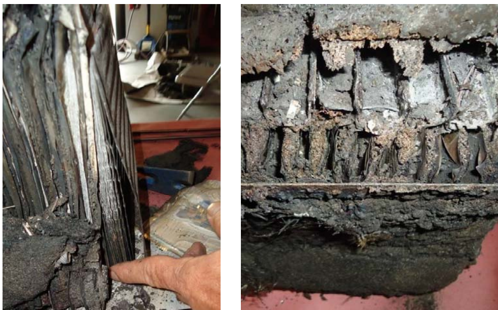
Figure 3.3-7. Typical Cell/Module Remains
