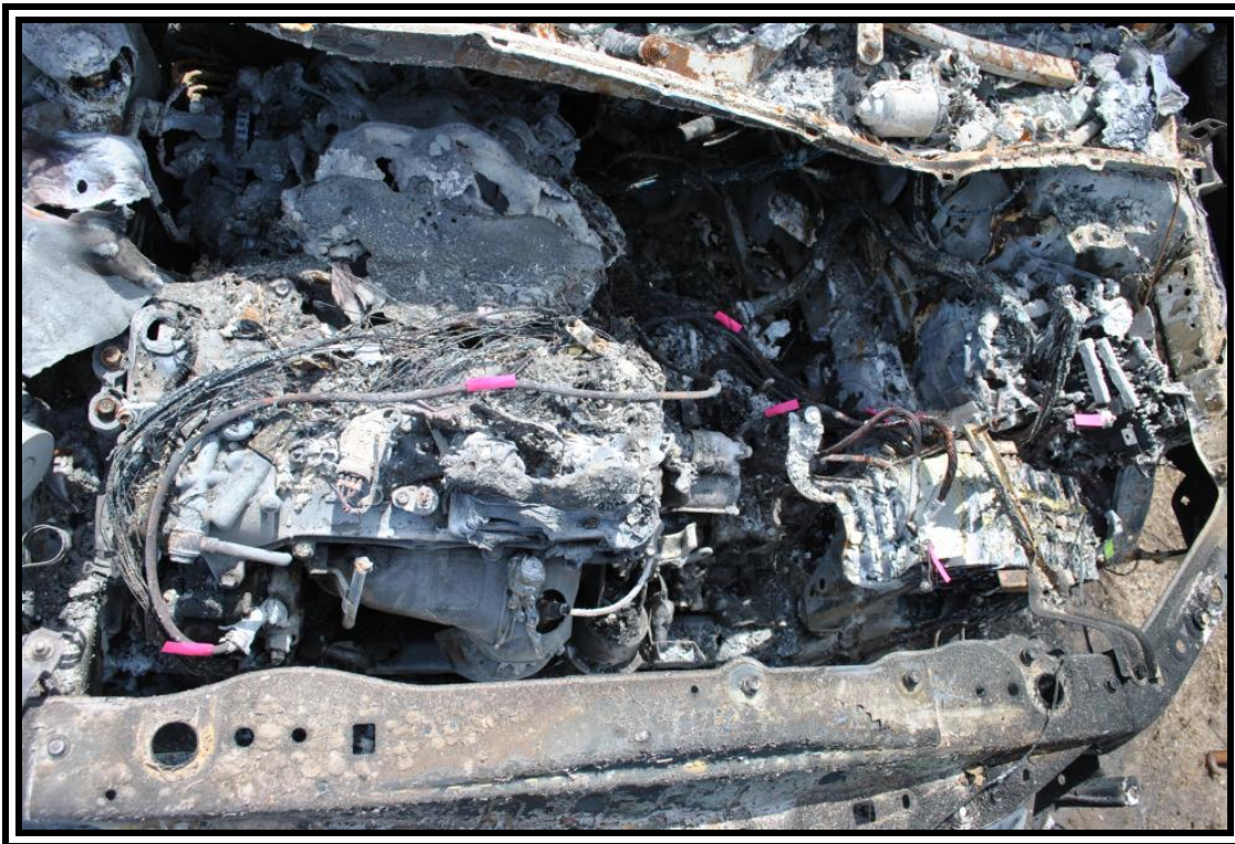
2011 Lexus RX350, +12vdc battery conductors
