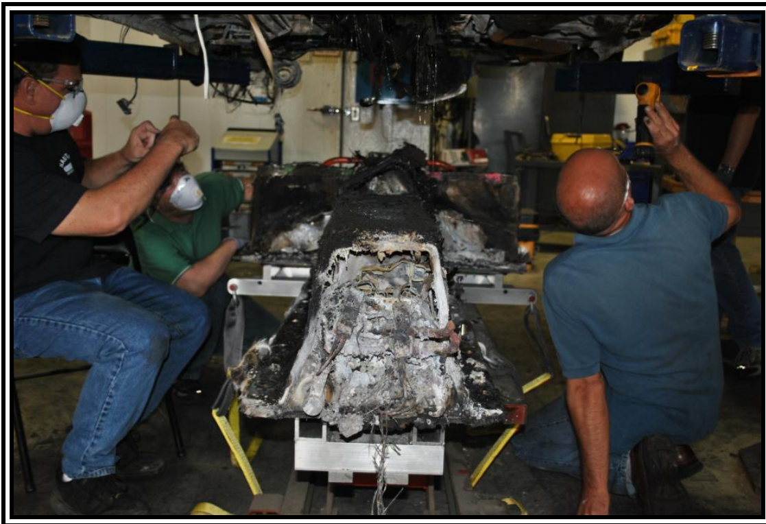
2011 Chevrolet Volt, high-energy battery pack removed from vehicle
