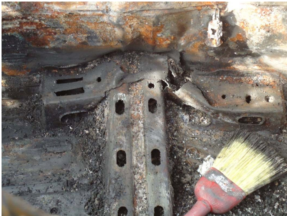
Figure 3.1-2. Crash Test Damage to the Outside of the Battery Compartment (Tunnel Section)
