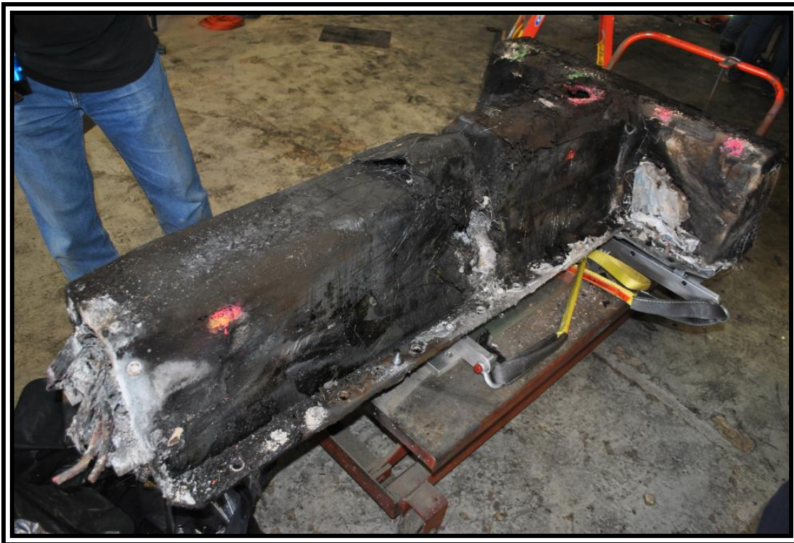
2011 Chevrolet Volt, driver's side of the high-energy battery pack
