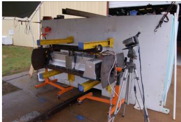
Figure 5.1 Thermocouples & Gas Detection Instrumentation connected to Battery
