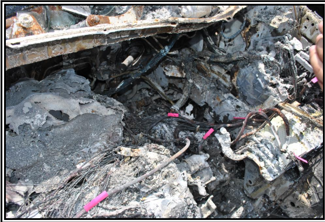
2011 Lexus RX350, +12vdc battery conductors
