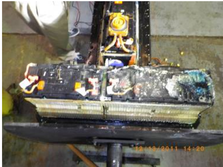
Figure 7.14 Fire Damage to Passenger Side End of Module 3
