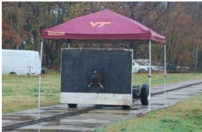
Figure 4.6 – Stinger attached to moving barrier face
