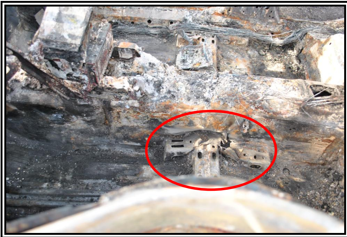
2011 Chevrolet Volt, driver's side interior showing impact intrusion into the center tunnel
