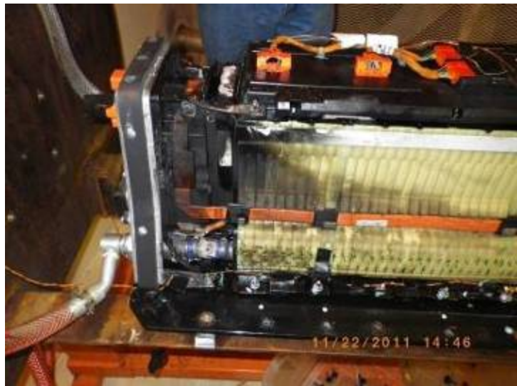
Figure 7.13 Arcing Damage to the Front of Module 1
