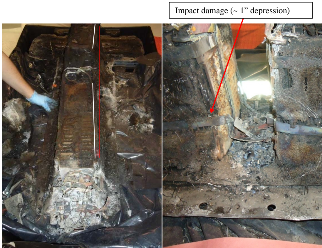
Figure 3.3-6. Physical Battery Damage
